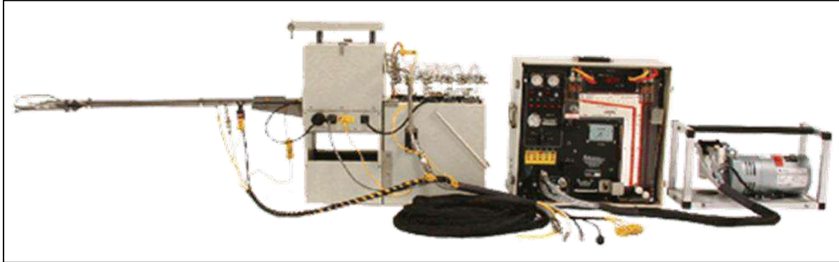
Figure 3: Full isokinetic sampling assembly
